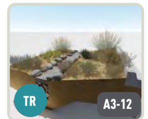
TR A3-12 INFILTRATION TRENCH
