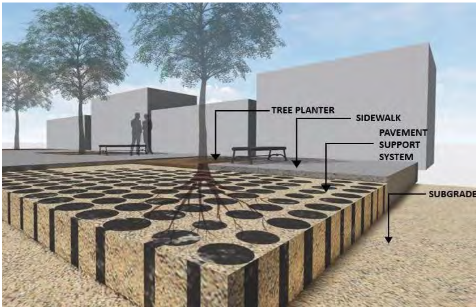
Tree planting in suspended pavement - ISOMETRIC VIEW.
