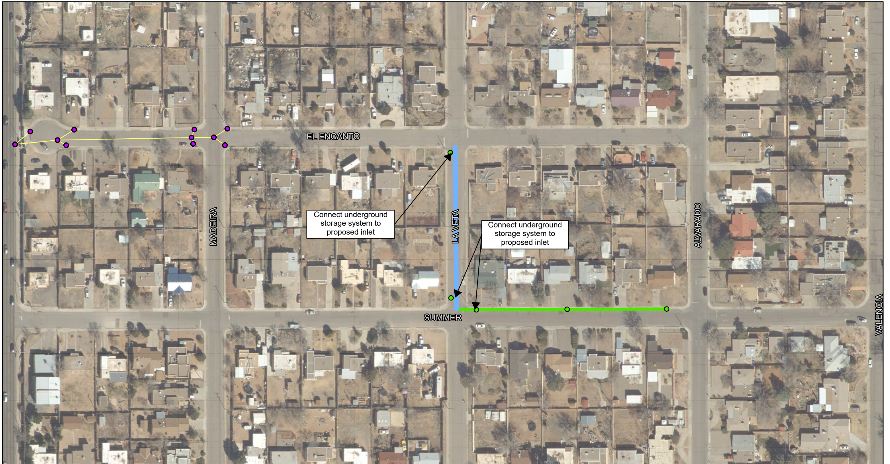
Pueblo Alto/Mile Hi GSI Phase IIIA 60% Design Figure 13 Proposed Underground System Mile Hi
