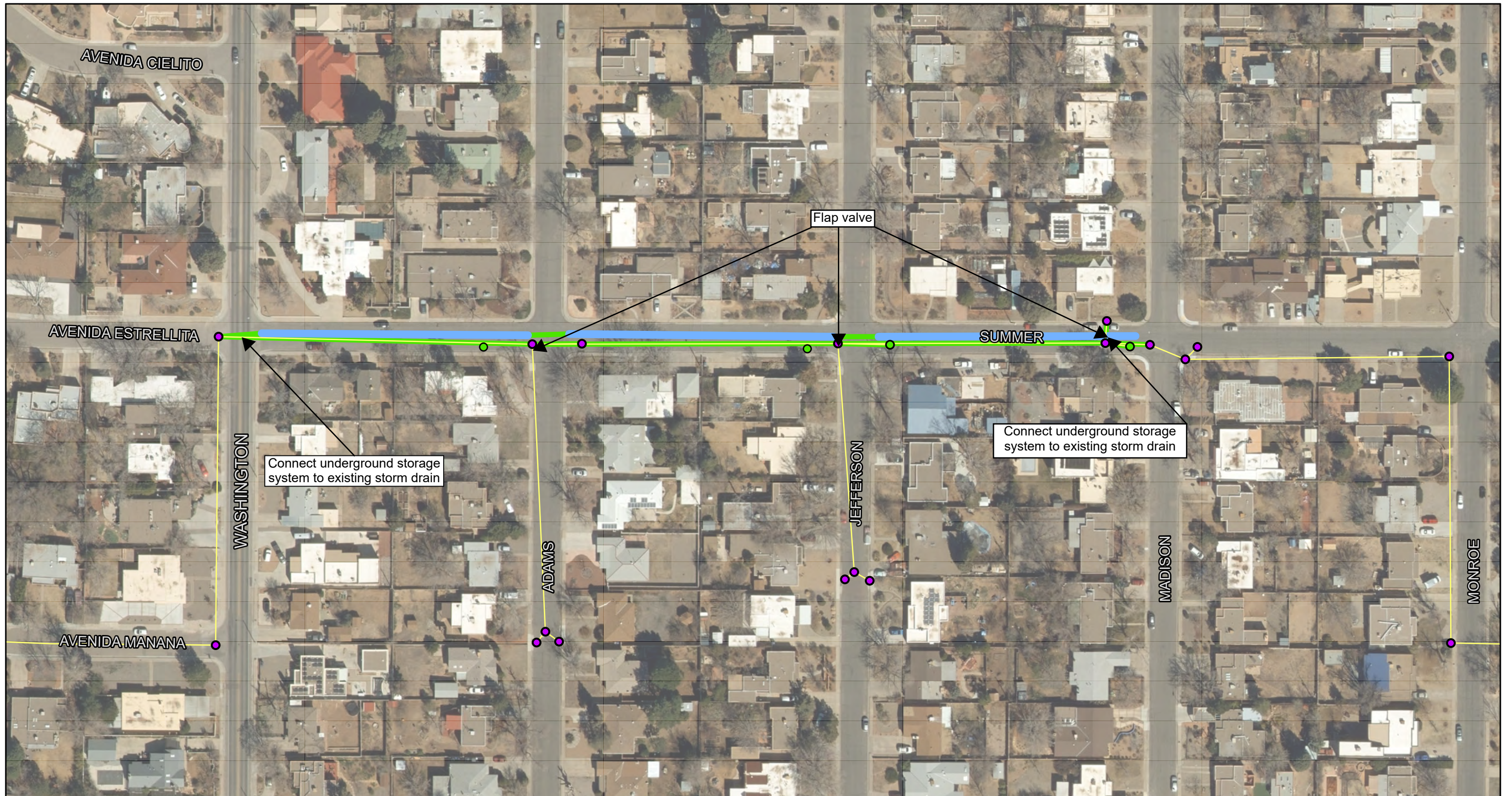
Pueblo Alto/Mile Hi GSI Phase IIIA 60% Design Figure 12 Proposed Underground System Pueblo Alto
